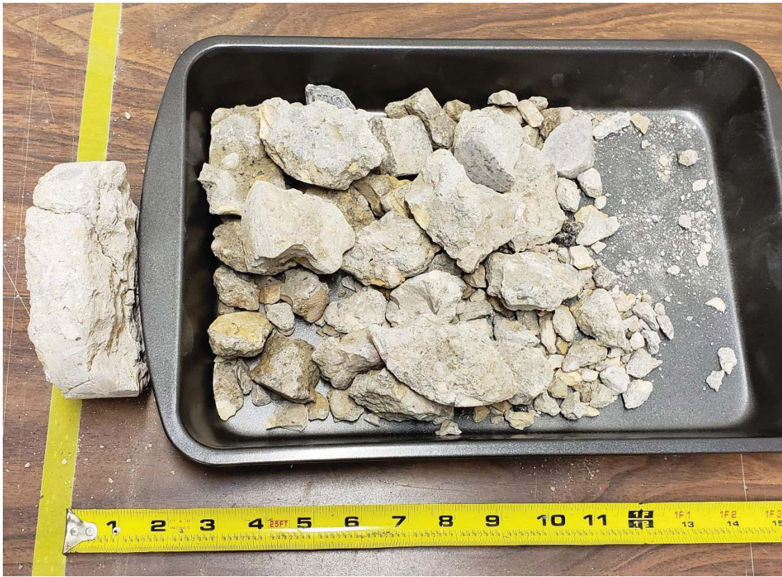
Figure 1 – PC-01 Maureen St (broken concrete shown, actual core size 150 mm)
